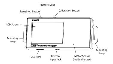
**Start/Stop Button:** Press this button for 3 seconds to start or stop logging data. This requires configuring the logger in HOBOware with a push button start or stop (see *Setting up the Logger*). You can also press this button for 1 second to record an internal event (see *Recording Internal Logger Events*) or to turn the LCD screen on if the option to turn off the LCD has been enabled (see *Setting up the Logger*).
