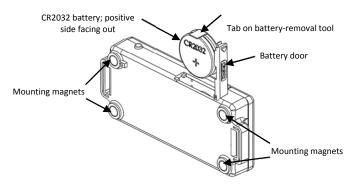
**WARNING:** Do not cut open, incinerate, heat above 85°C (185°F), or recharge the lithium battery. The battery may explode if the logger is exposed to extreme heat or conditions that could damage or destroy the battery case. Do not dispose of the logger or battery in fire. Do not expose the contents of the battery to water. Dispose of the battery according to local regulations for lithium batteries.
