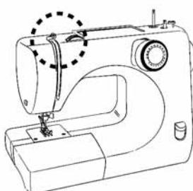
Support the thread on the sewing machine with one hand, using the other hand pass the thread around the thread guide as shown in the diagram.
